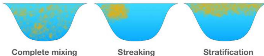
Figure 4: Illustration of how complete mixing, streaking or stratification affect the concentration in a river.
