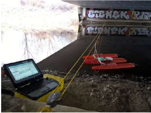
(c) Controlling index station with ADCP boat.
